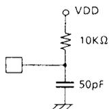
Serial port (completion of transmission)
