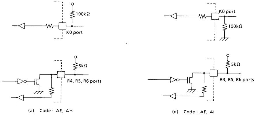
Figure 2. I/O code and external circuitry
