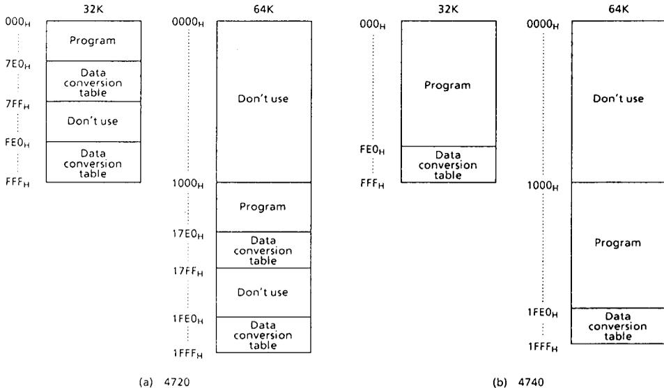
Figure 1. Capacity of EPROM and Program area
