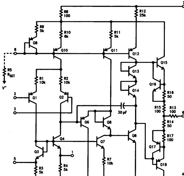
Figure 1: Functional Diagram
