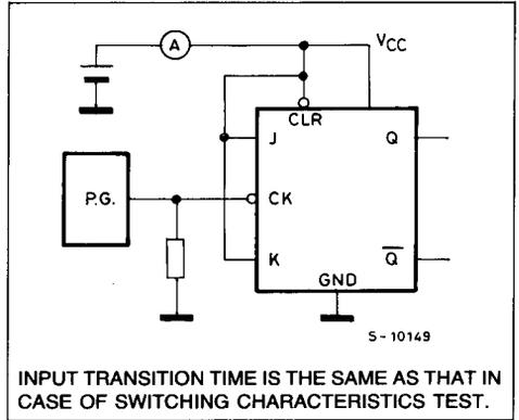
INPUT TRANSITION TIME IS THE SAME AS THAT IN CASE OF SWITCHING CHARACTERISTICS TEST.
