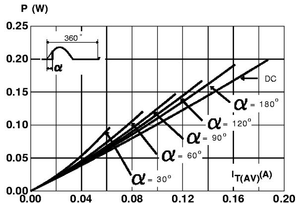
**Fig.2 :** Correlation between maximum average power dissipation and maximum allowable temperature (Tamb).
