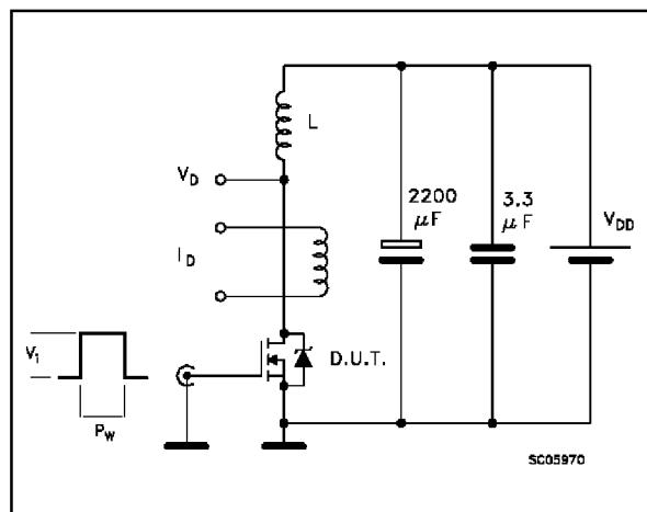
**Fig. 1:** Unclamped Inductive Waveform
