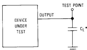
\*Includes all probe and jig capacitance.
