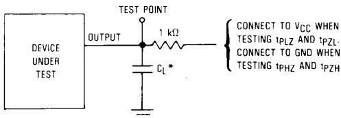
\*Includes all probe and jig capacitance.
