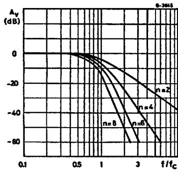
**Figure 12 : Amplitude Response ( ±1dB ripple)**
