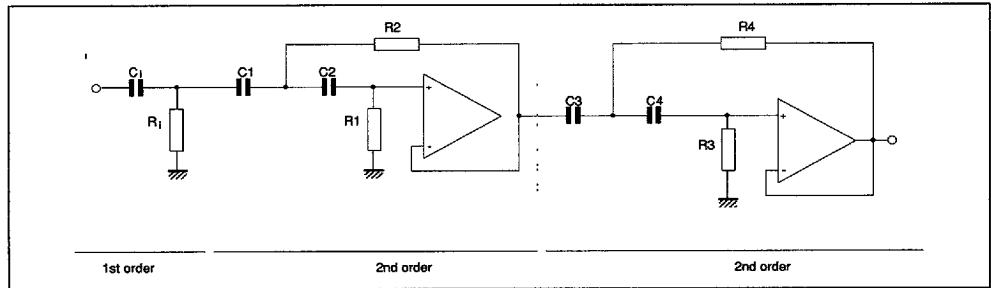
**Figure 17 : Multiple Feedback 8-pole Bandpass Filter**
