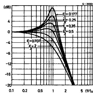
Three parameters are needed to characterize the frequency and phase response of a 2<sup>nd</sup> order active filter : the gain ( $G_v$ ), the damping factor ( $\xi$ ) or the Q-factor ( $Q = (2 \xi)^{-1}$ ), and the cut-off frequency ( $f_c$ ).
