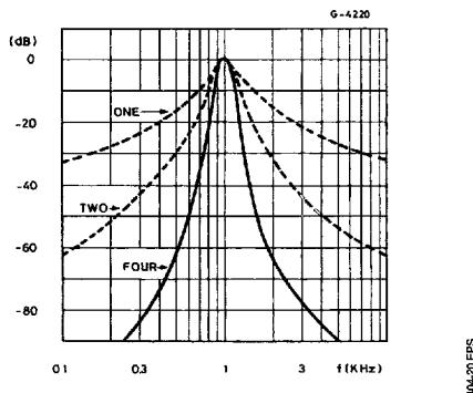
**Figure 19 : Bandwidth of Bandpass Filter**
