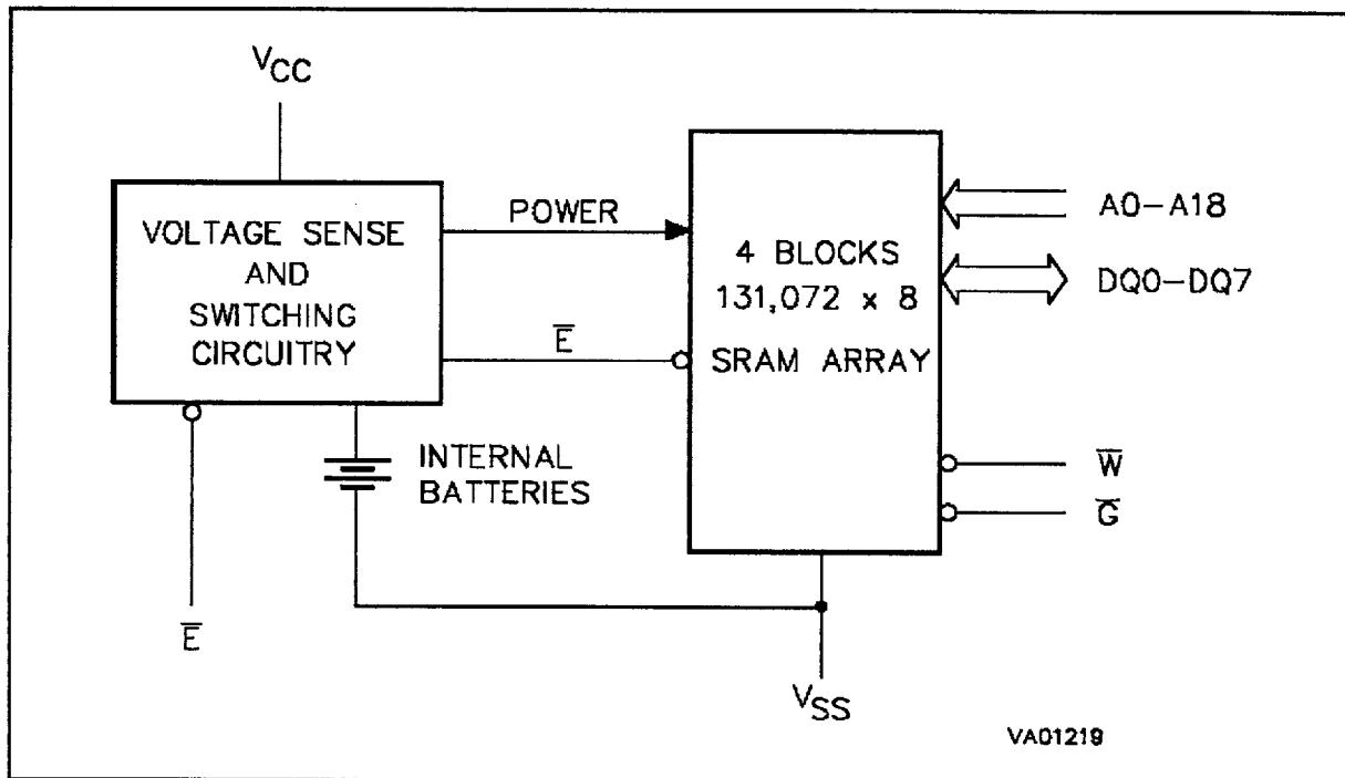
one of the 524,288 bytes of data is to be accessed. Valid data will be available at the Data I/O pins within  $t_{AVQV}$  (Address Access Time) after the last address input signal is stable, providing that the E and G (Output Enable) access times are also satisfied. If the E and G access times are not met, valid data will be available after the later of Chip Enable Access Time ( $t_{ELQV}$ ) or Output Enable Access Time ( $t_{GLQV}$ ).
