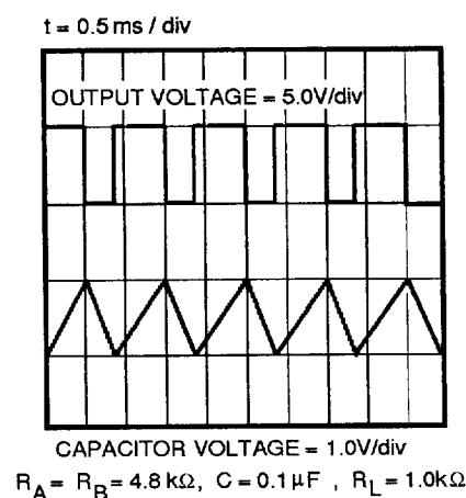
$R_A = R_B = 4.8 \text{ k}\Omega, C = 0.1 \mu\text{F}, R_L = 1.0 \text{k}\Omega$
