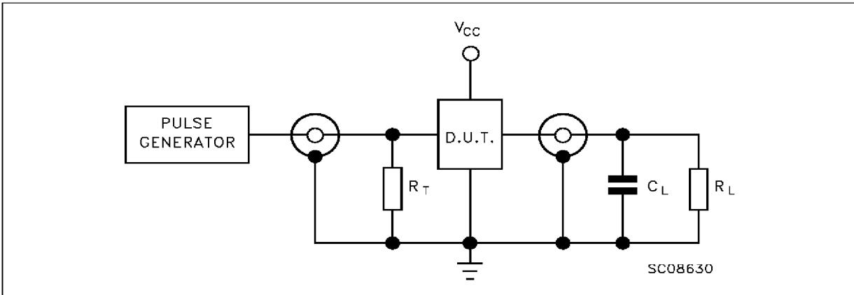
$C_L = 50 \text{ pF}$  or equivalent (includes jig and probe capacitance)
