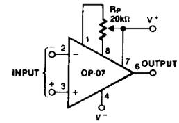
Figure 1. Offset Nulling Circuit
