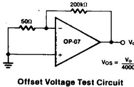
Offset Voltage Test Circuit
