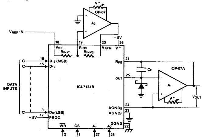
Figure 3. OP-07s Used for Reference Inversion and Voltage Output with ICL7134B DAC
