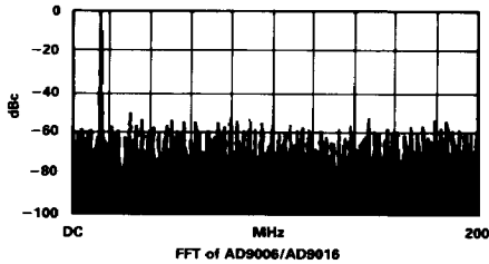
400MSPS: F_{IN} = 14.8\text{MHz} ; V_{IN} = 1.0\text{dB Below FS}
