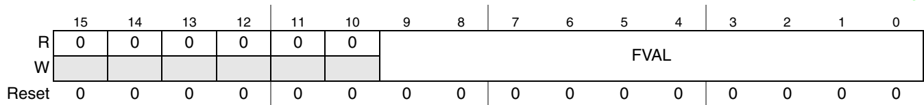
Figure 3-33. Sync Frame ID Acceptance Filter Value Register (SFIDAFVR)
