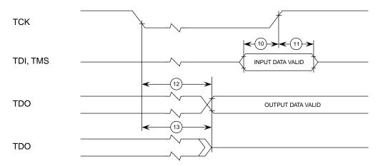
Figure 21. Test Access Port Timing Diagram
