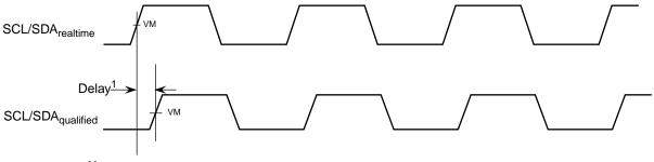
The delay is the local memory clock times DFFSR times 2 plus 1 local memory clock.
