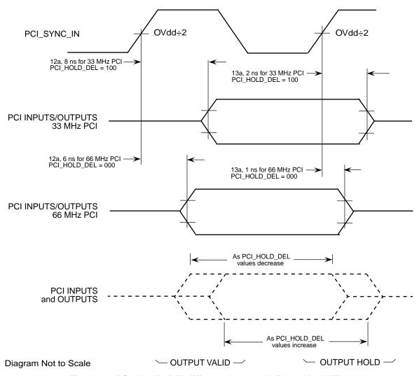
Figure 11. PCI\_HOLD\_DEL Effect on Output Valid and Hold Time
