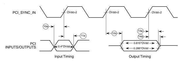
Figure 8. Input - Output Timing Diagram Referenced to PCI\_SYNC\_IN
