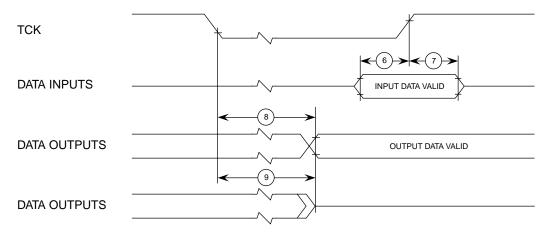
Figure 20. JTAG Boundary Scan Timing Diagram
