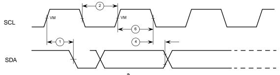
Figure 12. I<sup>2</sup>C Timing Diagram I
