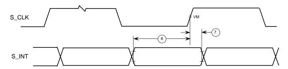
Figure 17. PIC Serial Interrupt Mode Input Timing Diagram
