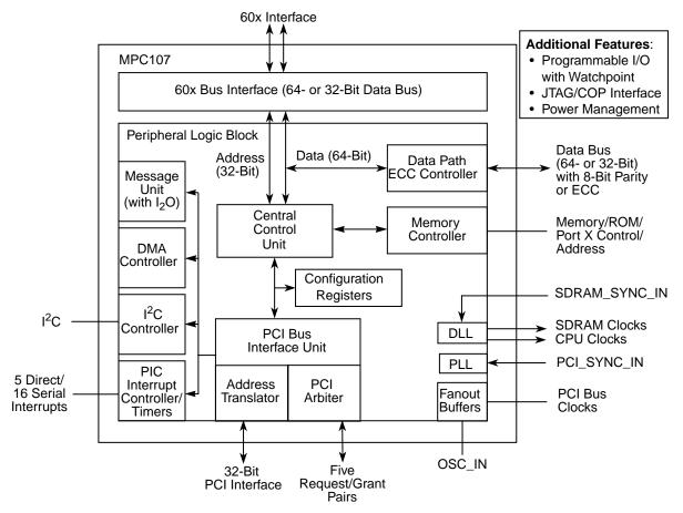
Figure 1. MPC107 Block Diagram
