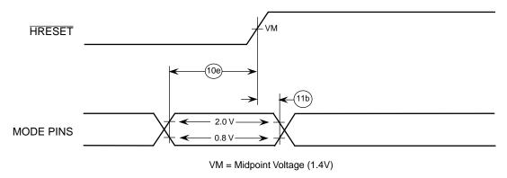
Figure 9. Input Timing Diagram for Mode Select Signals
