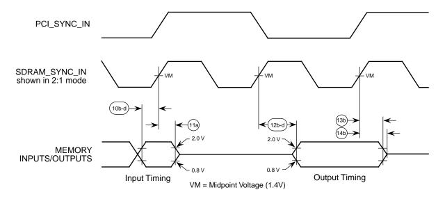
Figure 7. Input - Output Timing Diagram Referenced to SDRAM\_SYNC\_IN
