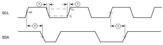
Figure 13. I<sup>2</sup>C Timing Diagram II
