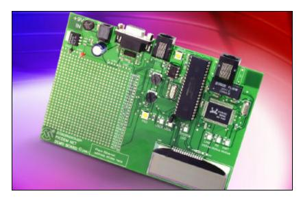
The PICDEM.net<sup>™</sup> demonstration board is an Internet/Ethernet demonstration board using the PIC16F877 microcontroller and TCP/IP firmware. The board supports any 40-pin DIP device that conforms to the standard pin out used by the PIC16F877 or PIC18C452.
