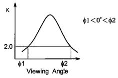
Contrast ratio K vs viewing angle  $\phi$
