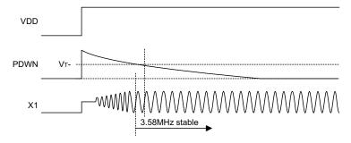
Note: reference  $C_1$ =0.1 $\mu$ F  $R_1$ =81 $k\Omega$
