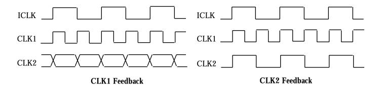
Using CLK1 as the feedback will always result in synchronized rising edges between ICLK and CLK1. But CLK2 could be a falling edge compared with ICLK. Therefore, wherever possible, we recommend the use of CLK2 feedback. This will synchronize the rising edges of all 3 clocks.
