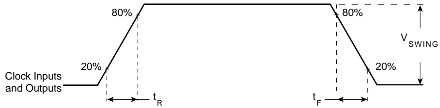
FIGURE 5 - INPUT AND OUTPUT RISE AND FALL TIME
