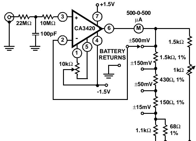
FIGURE 2. HIGH INPUT RESISTANCE VOLTMETER
