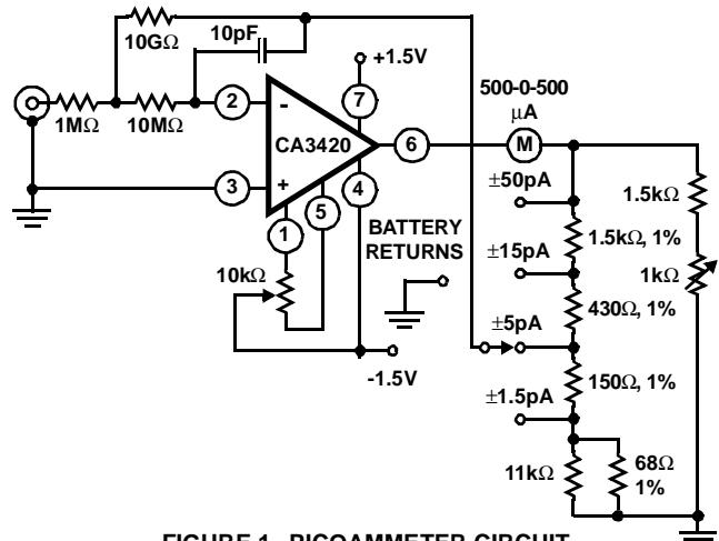
FIGURE 1. PICOAMMETER CIRCUIT
