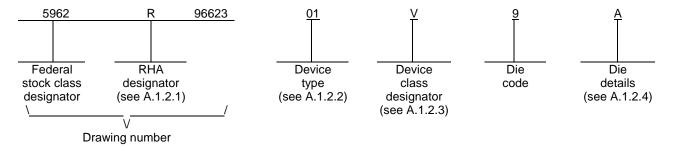
A.1.2.1 RHA designator. Device classes Q and V RHA identified die shall meet the MIL-PRF-38535 specified RHA levels. A dash (-) indicates a non-RHA die.
