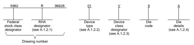
A.1.2.1 <u>RHA designator</u>. Device classes Q and V RHA identified die shall meet the MIL-PRF-38535 specified RHA levels. A dash (-) indicates a non-RHA die.
