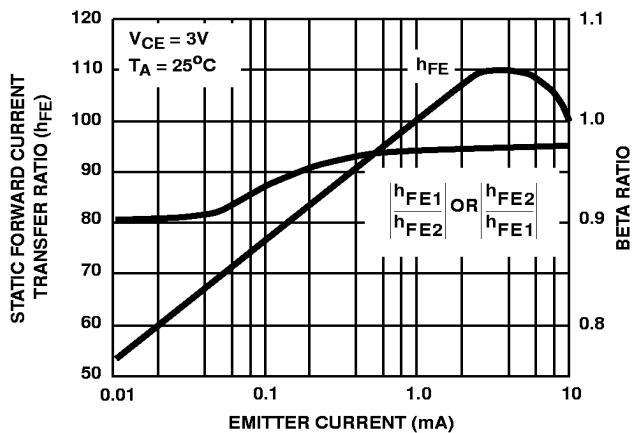
**FIGURE 3. TYPICAL STATIC FORWARD CURRENT TRANSFER RATIO AND BETA RATIO FOR Q<sub>1</sub> AND Q<sub>2</sub> vs Emitter Current**
