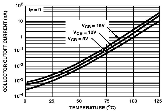
FIGURE 1. TYPICAL COLLECTOR-TO-BASE CUTOFF CURRENT
