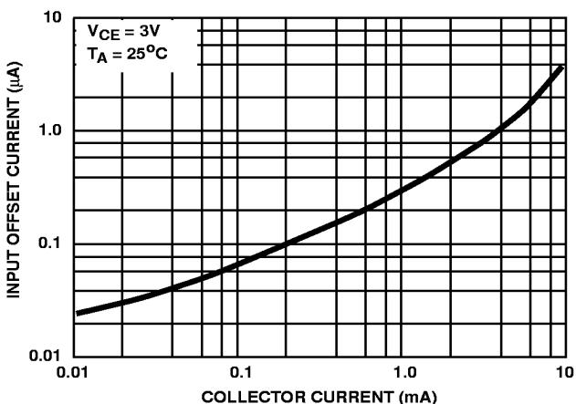
**FIGURE 4. TYPICAL INPUT OFFSET CURRENT FOR MATCHED TRANSISTOR PAIR Q<sub>1</sub>Q<sub>2</sub> vs COLLECTOR CURRENT**
