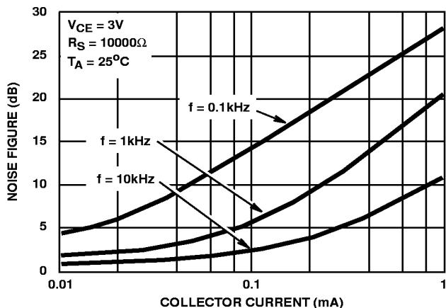
FIGURE 10. TYPICAL NOISE FIGURE vs COLLECTOR CURRENT
