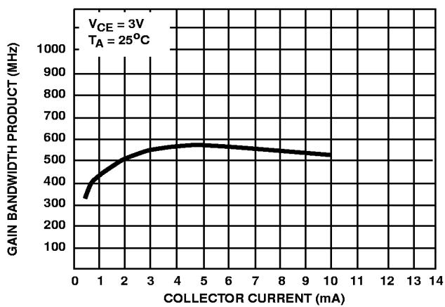
FIGURE 16. TYPICAL GAIN BANDWIDTH PRODUCT vs COLLECTOR CURRENT
