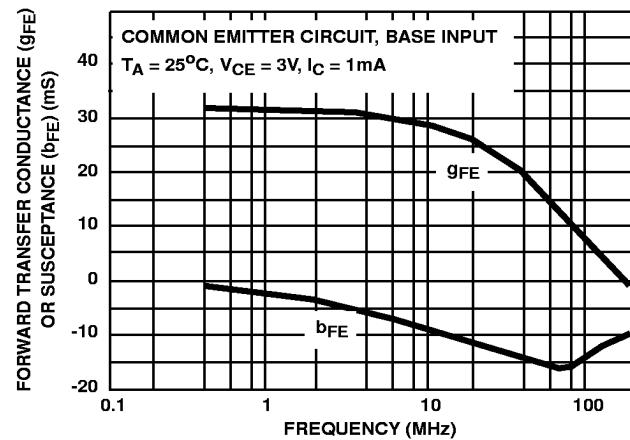
FIGURE 12. TYPICAL FORWARD TRANSFER ADMITTANCE vs FREQUENCY
