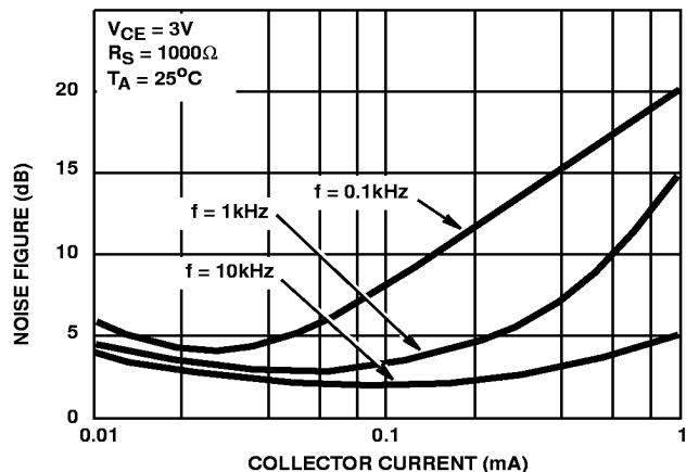
FIGURE 9. TYPICAL NOISE FIGURE vs COLLECTOR CURRENT
