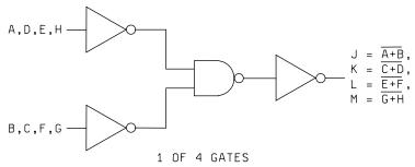
FIGURE 3. Logic diagrams.
