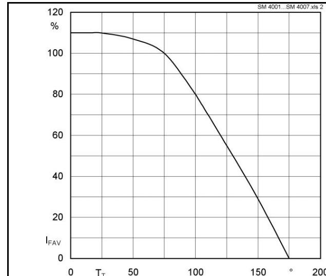
Fig. 2 Rated forward current vs. temp. of the terminals <sup>4)</sup>
