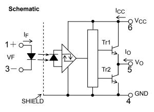
0.1 µF bypass capacitor must be connected between pins 6 and 4. Unit in mm
