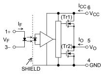
A 0.1  $\mu F$  bypass capacitor must be connected between pin 6 and 4. (See Note 6)
