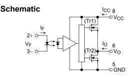
A 0.1  $\mu\text{F}$  bypass capacitor must be connected between pins 8 and 5. (See Note 6)
