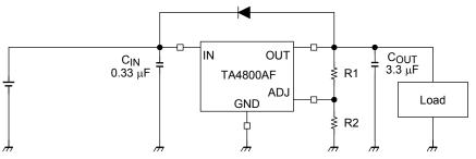
• There is a possibility that internal parasitic devices may be generated when momentary transients cause a terminal's potential to fall below that of the GND terminal. In such case, that the device could be destroyed. The voltage of each terminal and any state must therefore never fall below the GND potential.
