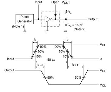
Note 1: Pulse width 50  $\mu s$  Duty cycle 10% Output impedance 50  $\Omega$   $t_{\Gamma} \le 5$  ns,  $t_{f} \le 10$  ns
