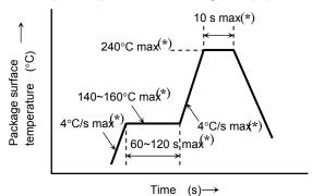
• The products are evaluated using above reflow soldering conditions. No additional test is performed exceed the condition (i.e. the condition more than (\*)MAX values) as a evaluation. Please perform reflow soldering under the above conditions.
