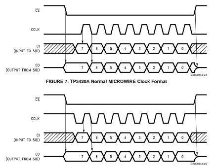
FIGURE 8. TP3420A Alternate MICROWIRE Clock Format
