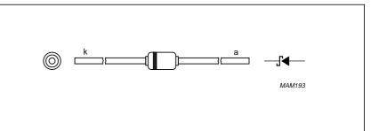
Fig.1 Simplified outline (SOD68; DO-34), pin configuration and symbol.
