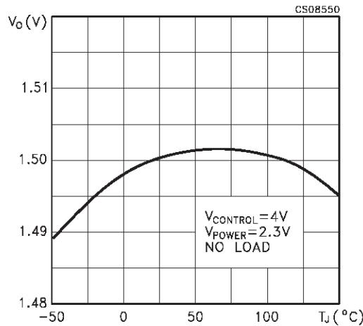
**Figure 2 : Minimum  $V_{\text{CONTROL}}$  Voltage vs Temperature**
