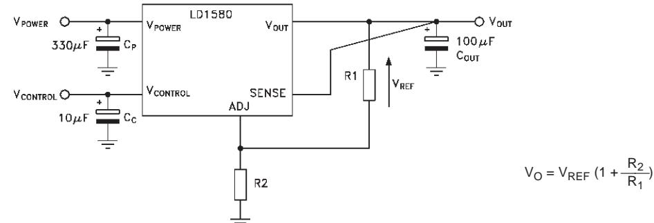
**ELECTRICAL CHARACTERISTICS FOR LD1580xx15 (  $T_j = -40^{\circ}\text{C}$  to  $125^{\circ}\text{C}$ ,  $C_P=330\ \mu\text{F}$ ,  $C_C=10\ \mu\text{F}$ ,  $C_{\text{OUT}}=100\ \mu\text{F}$ , unless otherwise specified)**
