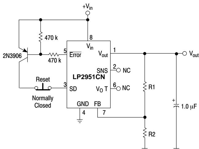
Error flag occurs when  $V_{in}$  is too low to maintain  $V_{out}$ , or if  $V_{out}$  is reduced by excessive load current.
