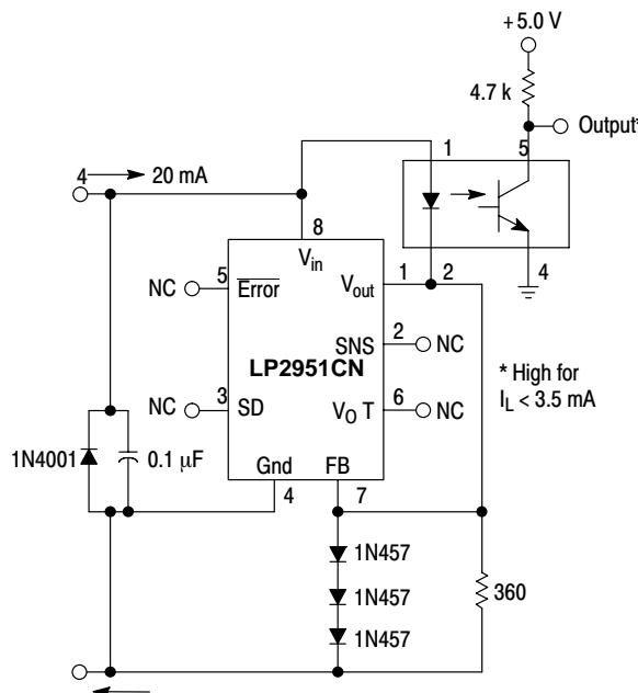
Figure 26. Open Circuit Detector for 4.0 to 20 mA Current Loop
