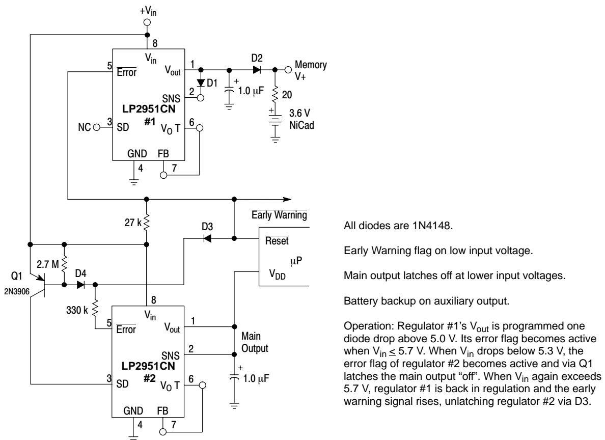
Figure 24. Regulator with Early Warning and Auxiliary Output
