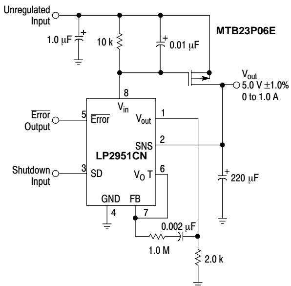
**Figure 19. 1.0 A Regulator with 1.2 V Dropout**
