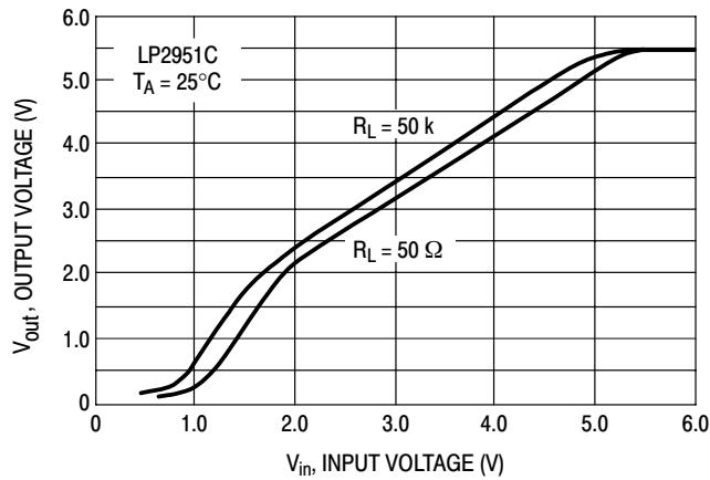
Figure 3. Dropout Characteristics
