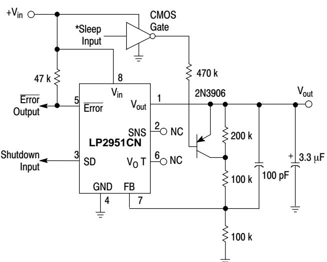
Figure 23. 5.0 V Regulator with 2.5 V Sleep Function
