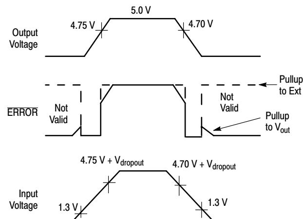
Figure 17.  $\overline{\text{ERROR}}$  Output Timing
