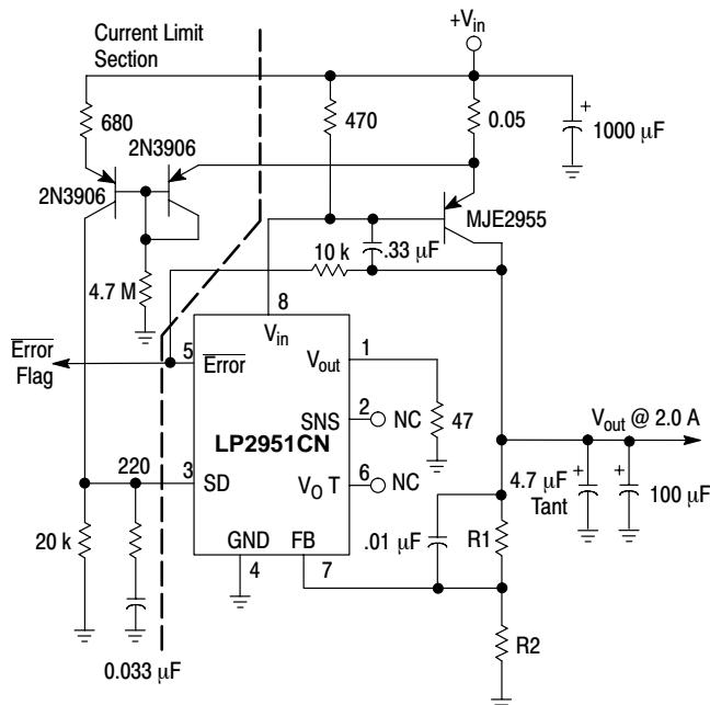
Figure 25. 2.0 A Low Dropout Regulator
