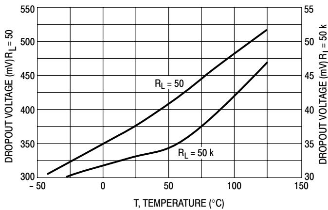
Figure 7. Dropout Voltage versus Temperature
