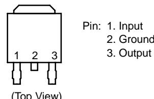
Heatsink surface (shown as terminal 4 in case outline drawing) is connected to Pin 2.
