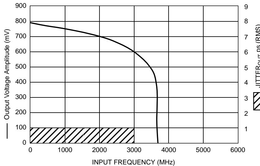
**Figure 3. Output Voltage Amplitude / RMS Jitter vs.
