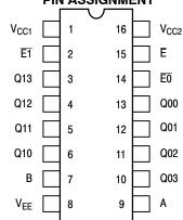
Pin assignment is for Dual-in-Line Package.
