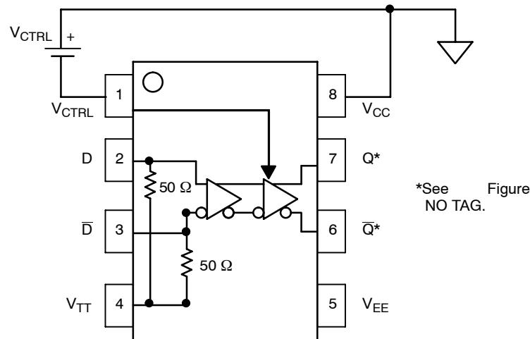
**Figure 4. Voltage Source Implementation,  $V_{CTRL}$  Pin 1**
