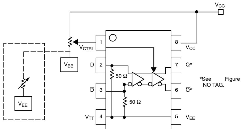
**Figure 5. Alternative Implementations,  $V_{CTRL}$  Pin 1**
