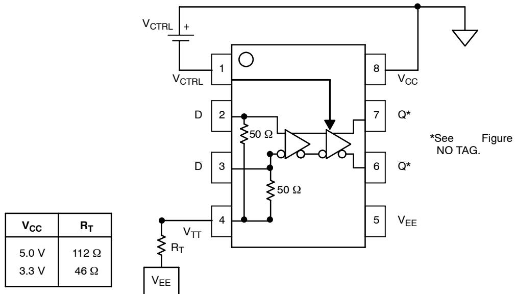
Figure 7. Alternate “Y” Termination Method, V<sub>TT</sub> Pin 4
