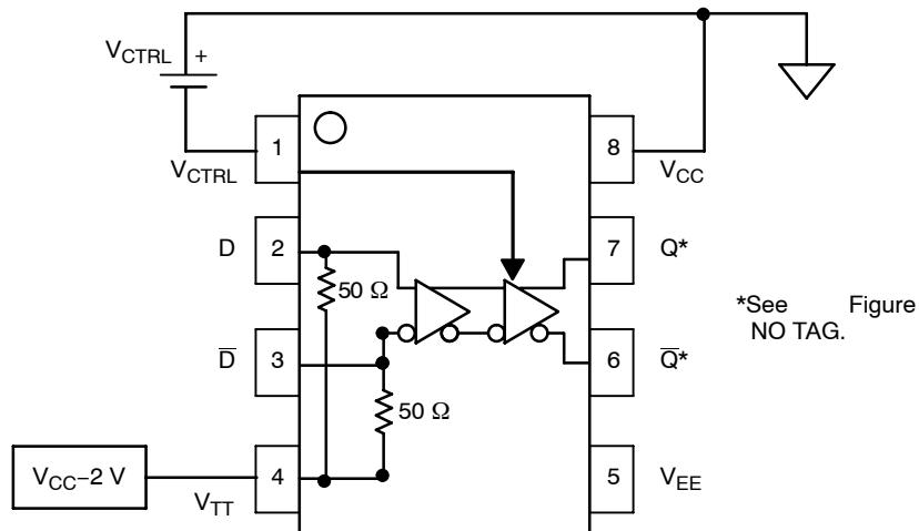
**Figure 6. Standard Termination Method,  $V_{TT}$  Pin 4**
