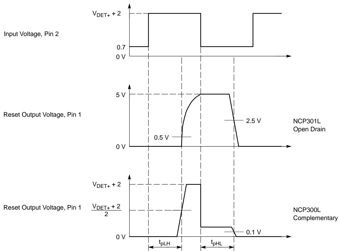
NCP300 and NCP301 series are measured with a 10 pF capacitive load. NCP301 has an additional 470 k pull-up resistor connected from the reset output to +5.0 V. The reset output voltage waveforms are shown for the active low 'L' devices. The upper detector threshold,  $V_{DET+}$  is the sum of the lower detector threshold,  $V_{DET-}$  plus the input hysteresis,  $V_{HYS}$ .
