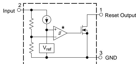
\* The representative block diagrams depict active low reset output 'L' suffix devices. The comparator inputs are interchanged for the active high output 'H' suffix devices.
