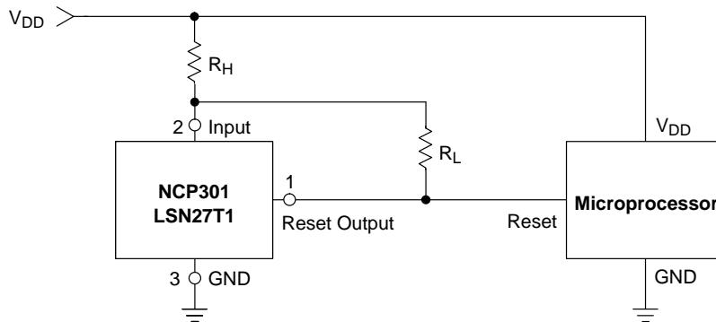
**Figure 26. Microprocessor Reset Circuit with Additional Hysteresis**
