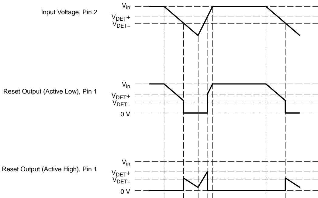
**Figure 21. Timing Waveforms**
