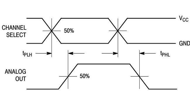
**Figure 9a. Propagation Delays, Channel Select to Analog Out**
