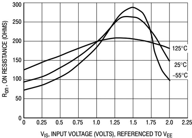
Figure 1a. Typical On Resistance, V<sub>CC</sub> - V<sub>EE</sub> = 2.0 V
