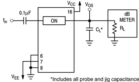
Figure 6. Maximum On Channel Bandwidth, Test Set-Up
