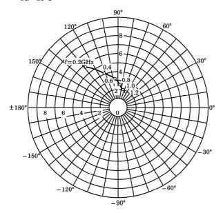
$\begin{array}{l} S_{22e} \\ V_{CE} = 10V \\ I_{C} = 2mA \\ Ta = 25^{\circ}C \\ (UNIT:\Omega) \end{array}$ j50 j25 j100 j150 j250 j10 <del>|</del>| 100 10 250 f=0.2GHz-j250 2′0.6 -j150 -j100 -j50
