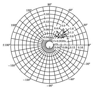
$\begin{array}{l} S_{21e} \\ V_{CE} = 10V \\ I_{C} = 5 \text{mA} \\ Ta = 25 ^{\circ}\text{C} \end{array}$
