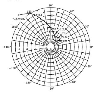
$\begin{array}{l} S_{22e} \\ V_{CE}\!=\!10V \\ I_{C}\!=\!5\text{mA} \\ T_{a}\!=\!25^{\circ}\!C \\ (U\text{NIT}:\Omega) \end{array}$
