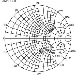
$\begin{array}{l} S_{11e} \\ V_{CE} \! = \! 10V \\ I_{C} \! = \! 20\text{mA} \\ T_{a} \! = \! 25^{\circ}\! C \\ (UNIT:\Omega) \end{array}$
