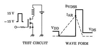
$$\begin{aligned} &RG = 25~\Omega \\ &V_{DD} = 25~V,~L = 428~\mu H \end{aligned} \qquad EAS =$$
