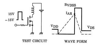
$$\begin{split} R_G &= 25~\Omega \\ V_{DD} &= 50~V,~L = 3.3~mH \end{split}$$
