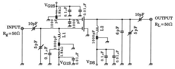
L1: 1 mm $\phi$  Ag plated copper wire, 2 turns, 8 mm ID
