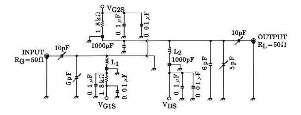
$L_1$ : 1 mm $\phi$  Ag plated copper wire, 2 turns, 8 mm ID
