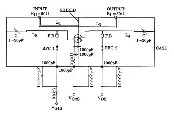
L<sub>1</sub>~L<sub>4</sub>:  $\phi$ 0.8 mm silver plated copper wire
