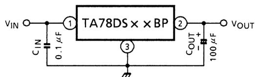
Capacitor  $C_{IN}/C_{OUT}$  must be guaranteed to operate of the temperature range that the regulator should be operated correctly, 100  $\mu\text{F}$  is a suitable value to suppress the oscillation phenomenon at the output terminal.
