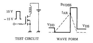
$$\begin{array}{l} T_{ch} = 25^{\circ}C \ (Initial) \\ Peak \ I_{AR} = 5 \ A, \ R_G = 25 \ \Omega \\ V_{DD} = 24 \ V, \ L = 1.0 \ mH \end{array} \\ \begin{array}{l} E_{AS} = \frac{1}{2} \cdot L \cdot I^2 \cdot \ (\frac{B_{VDSS}}{B_{VDSS} - V_{DD}}) \end{array}$$
