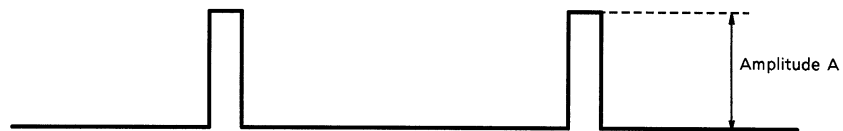
Fig.C Test signals for TA1310ANG chroma, color difference, and Y stage
